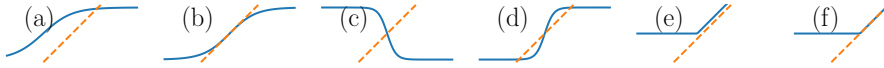
Figure 2: (Blue) Layers (1) on the interval [-1, 1] when Y = 0 , (Orange) identity. (a) \tanh(0.9z+2) has derivative \leq 0.9 so it admits a unique fixed point. (b) \tanh(z) has derivative \leq 1 . It satisfies the conditions of Proposition 2 on (-1, 0) and (0, 1) and so admits a unique fixed point. (c) \tanh(-3z) is not a contraction but admits a unique fixed point; contractions are not necessary. (d, e, f) \tanh(3z) , \text{ReLU}(z + 0.2) , \text{ReLU}(z) are not contractions and admit 3, 0 and uncountably many fixed points.
